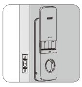
Install reinforcement plate and strike into door jamb.
