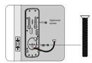
Attach cable assembly to the interior assembly PCB by lining up notches on top of cable connector to slots on PCB connector. Press connector in firmly until completely connected.
