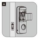
Keep your lock in "unlock"status, insert 4x AA hatteries in battery pack.
