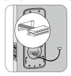
6. Secure both assemblies using the screws provided. Make sure the exterior assembly is vertically aligned. If you added the cross bolt, securely tighten the post to the exterior Ease unit with the additional screw provided.
