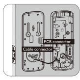
8. Install interior assembly on inside mounting plate.
